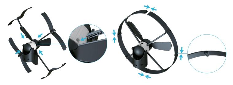
3.Remove the Energy Treasure decorative ring, align the unlocking mark of the Energy Treasure with the triangular mark on the fan installation interface, and rotate to connect. When the locking mark on the Energy Treasure is aligned with the triangular mark on the fan, the installation is successful.
